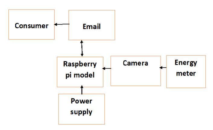
Figure 8. The Block Diagram of IOT based Energy Meter
