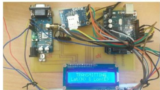
Figure 5. GSM module transmitting the latitude and Longitude of the vehicle's location.
