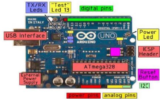
Figure 2. Arduino Uno Atmega328 microcontroller board
