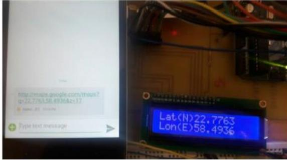
Figure 6. Extracted latitude and longitude send to the specific mobile number as Google maps link.
