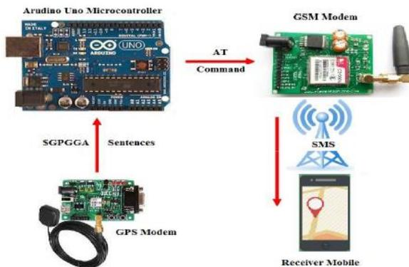
Figure 1. Block diagram of tracking and accident detection system based on GSM and GPS technology
