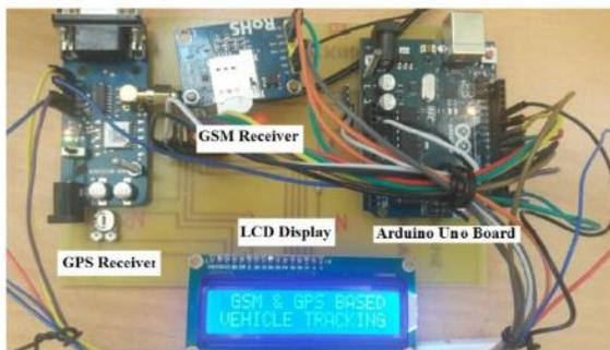
Figure 4. Status of the system when it is powered up
