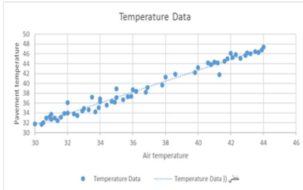
Figure 1: The air temperature and surface asphalt pavement temperature during April month.
