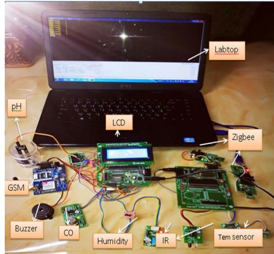
Figure 4: Real time system of Industrial monitoring system
