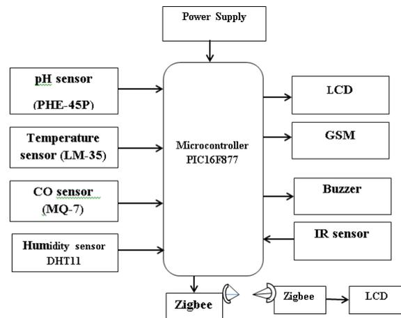
Figure 1: shows the block diagram of the system
