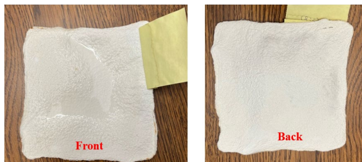
Figure 12. Water resistance test for crosslinked wastepaper pulp/alginate film. Left: Top side of the film loaded with water. Right: Bottom side of the film. No water has passed through.
