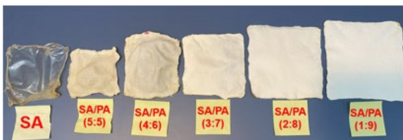
Figure 6. Photograph of wastepaper pulp/alginate agricultural mulch films synthesized using different SA/PA ratios, all of which were crosslinked with \text{Ca}^{2+} ions. In the photograph, the amount of wastepaper pulp increases from left to right. The SA/PA (2:8, wt%) and SA/PA (1:9, wt%) films experienced the least shrinkage and warpage.
