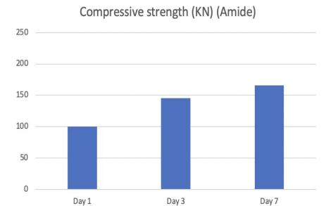
The compressive strength of BPA epoxy resin cured with Amide hardener showed an increase of 45.1% on day 3 and an increase of 65.4% on day 7. Amide hardener shows the greatest rate of change among all tested hardeners.
