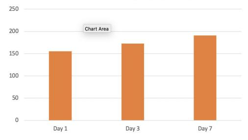
The compressive strength of BPA epoxy resin cured with TETA hardener showed an increase of 11.1% in compressive strength on day 3 and an increase of 23% on day 7. Teta hardener showed the second greatest initial and final compressive strength and exhibits the least rate of change among all tested hardeners.
