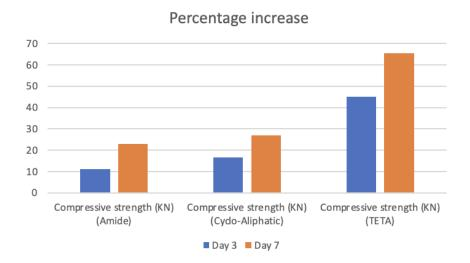
The experiments demonstrated that each hardener had a similar impact on the material's performance, increasing it drastically with similar slopes over a period of time. The TETA hardener exhibited notable compressive strength on day 1. Amide hardener exhibited the least compressive strength on day 1, but showed the greatest difference from day 1 to day 7 in compressive strength. The cyclo-aliphatic epoxy resin showed the greatest initial and final compressive strength.
