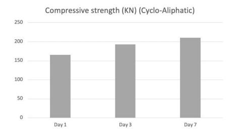
The compressive strength of BPA epoxy resin cured with Cyclo-Aliphatic hardener showed an increase of 16.6% on day 3 and an increase of 27% on day 7.
