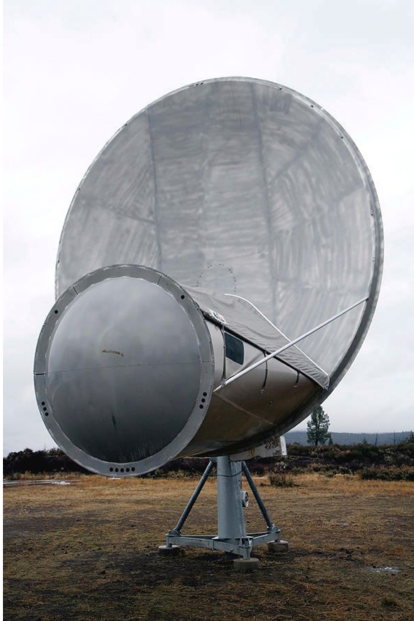
Figure 3. The Allen Telescope Array (ATA) is a radio telescope array dedicated to astronomical observations and a simultaneous SETI. The ATA is a centimeter-wave array at the Hat Creek Radio Observatory, California. Compared to a large dish antenna, large numbers of smaller dishes are cheaper for the same collecting area. To get similar sensitivity, the signals from all telescopes must be combined. https://sciencephotogallery.com/featured/allen-telescope-array-adam-hart-davisscience-photo-library.html
