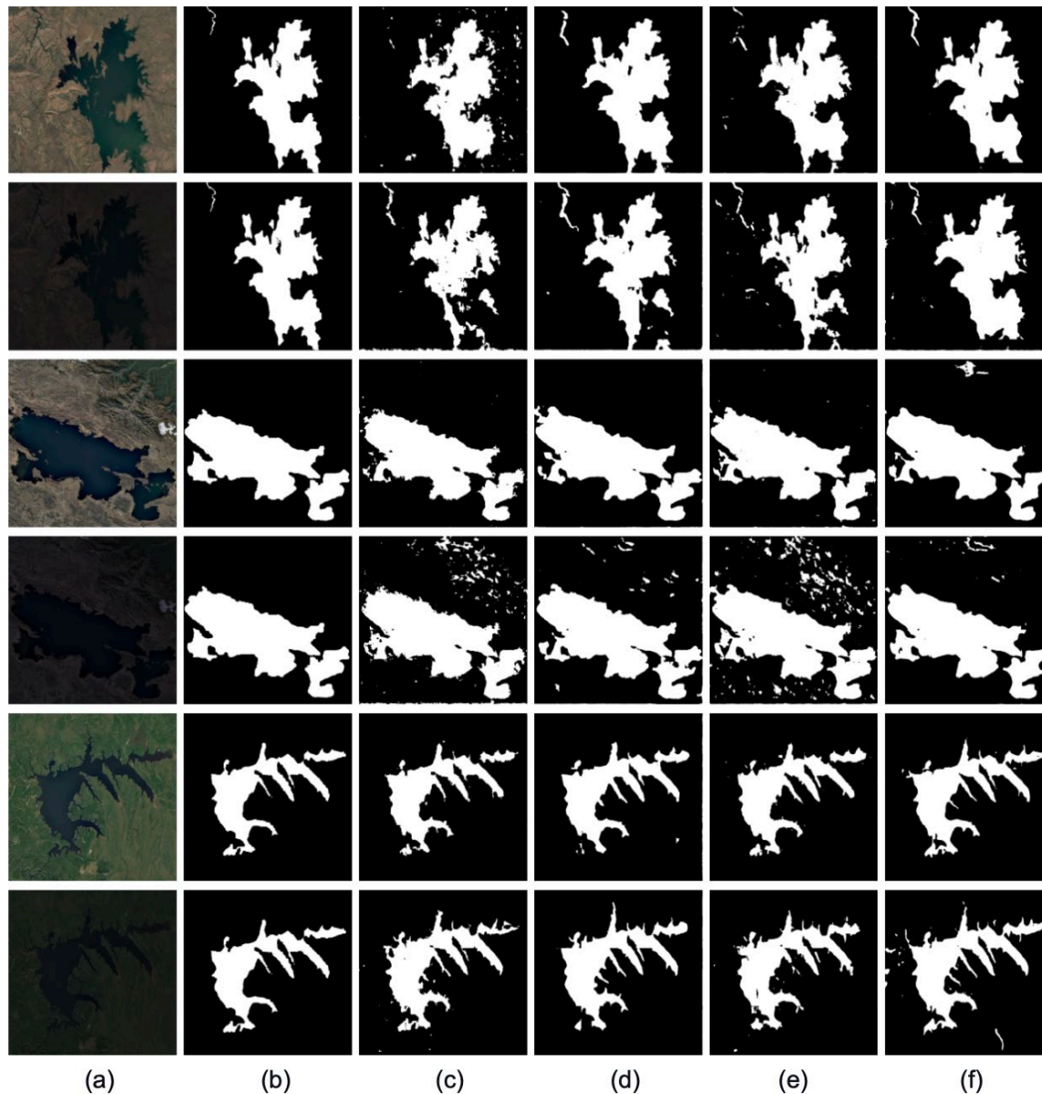
Figure 6. Performance Comparison of Segmentation Models with Our Dataset. (a) Images, (b) Ground-truth, (c) FCN, (d) U-Net, (e) Link-Net (f) DeepLabsV3+
