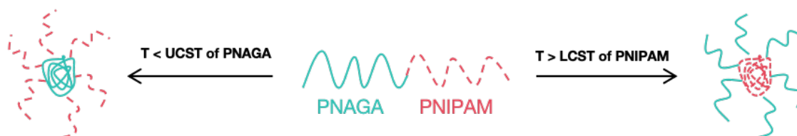
Figure 5. LCST/UCST behavior of thermo-responsive polymers.
