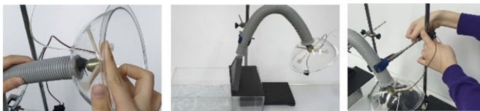
Figure 29. Final step to make the cooling fan by ensuring it with the support of a stand
