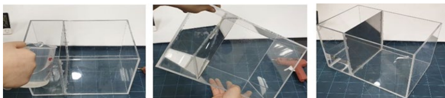
Figure 11. Checking to see if there is any water leakage by pouring and tilting the acrylic box
