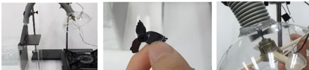
Figure 30. Testing the efficiency of a gas range hood device model and the hemispherical cooling fan
