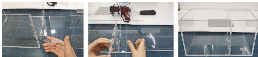
Figure 9. Making containers using acrylic plates and combining them together with acrylic glue
