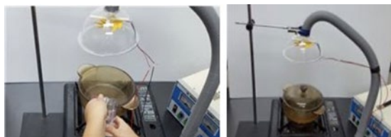
Figure 31. Testing to verify the ability of the hemispherical cooling fan to intake hot air using Bernoulli's principle
