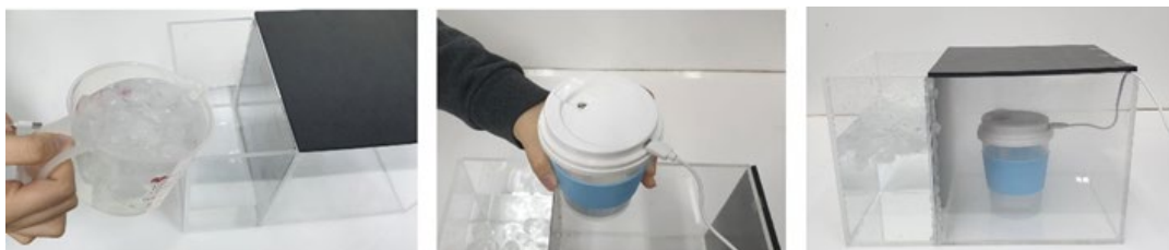
Figure 12. Creating a condensation trap using ice water and humidifier in the opposite sides with the black woodlock covering top
