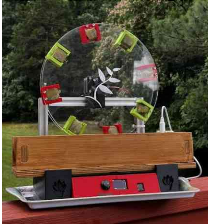
Figure 13. Functioning Rotary Hydroponic Garden System
