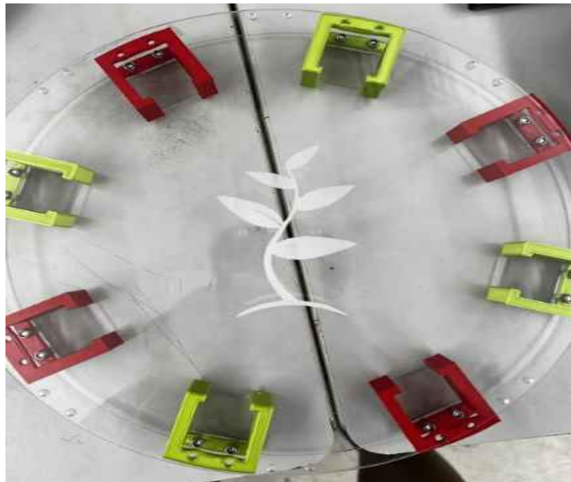
Figure 8. Cube Holders Attached to Outer Casing
