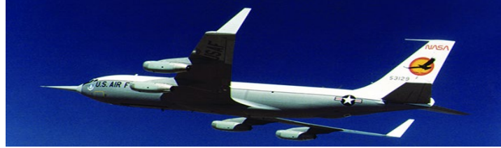
Figure 1. KC-135A fitted with winglets. [9]NASA, O., 1979, KC-135A in flight - winglet study, In Flight.
