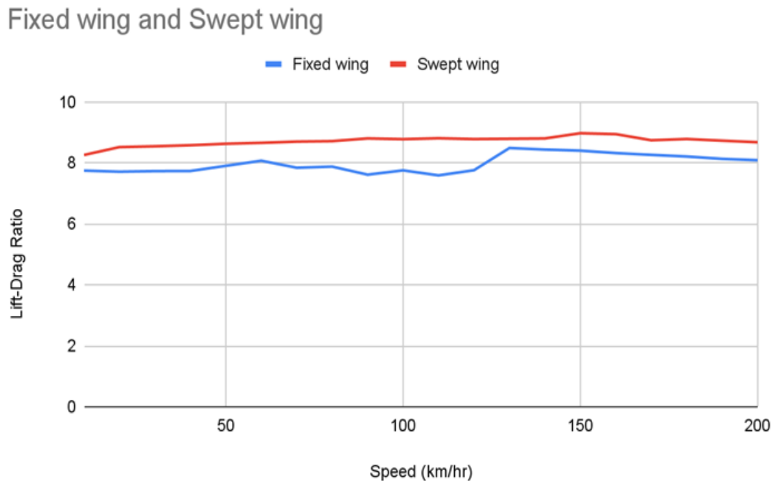
Figure 2. Lift to drag ratio (dimensionless) for the two wing designs as a function of the airspeed. Throughout the range of speeds considered, the swept wing has a superior lift to drag ratio.
