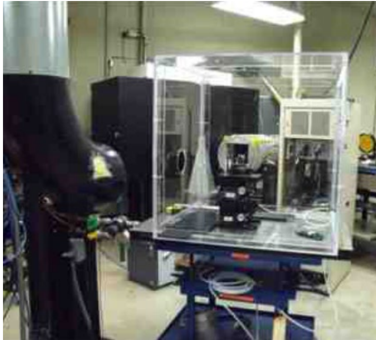
Figure 4. Plexiglass test box for containment of test materials within inert atmosphere used at the LHMEI. This figure was originally published by Sepka et al. in the proceedings for the 36th International Conference and Expo on Advanced Ceramics and Composites [16]
