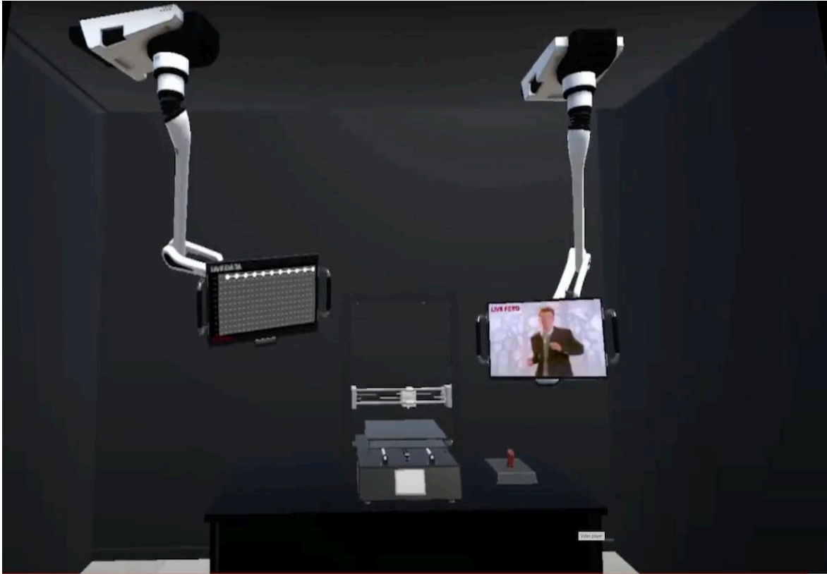
Figure 4. The VR scene displaying the 3D-printer, sensor data display, and video monitor.
