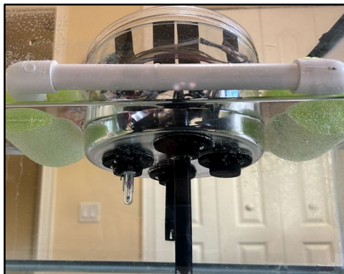
Figure 4. Verifier – Completed Verifier floatation system placed in the pond simulator.
