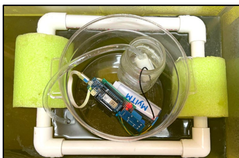
Figure 5. Destroyer system engineered with a submersible pump and electronics for remote algal mitigation.
