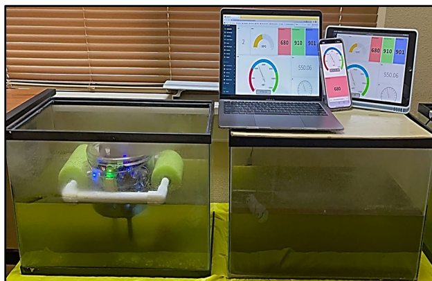
Figure 7. Lab Analysis Testing (LAT) – Full H&S system showing floatation device in pond simulator transmitting real-time algal parameter metrics to computer and handheld devices.
