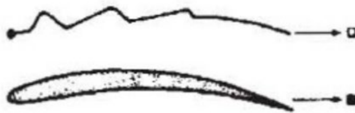
Figure 2. Top: corrugated wing cross section of a hoverfly. Bottom: smooth counterpart cross section made by drawing an “envelope” around the corners of the corrugations (Rees, 1975a).
