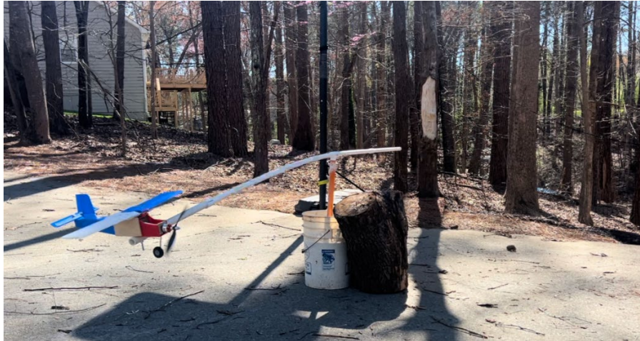
Figure 13. MAV Experiment Setup in Turbulent Atmospheric Layer. Above is the setup for the flight time/speed experiments made of PVC pipes. A log was placed on the 5-gallon bucket to stabilize the system during flight trials.
