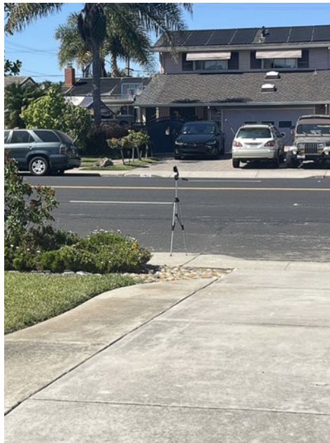
Figure 2. Camera mounted on a tripod 1.5m off the pavement. This setup allowed us to capture testing footage for our model and simulate the effectiveness at an average biker's height.
