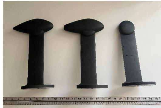
Figure 5. Fairings tested in the water channel. From left to right: 0%H, 30%H, control wheel.
