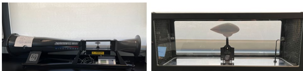
Figure 4. Jet Stream 500 wind tunnel and testing setup.
