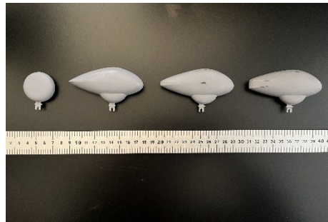
Figure 3. Fairings tested in the wind tunnel. From left to right: control wheel, 0%H, 15%H, 30%H.
