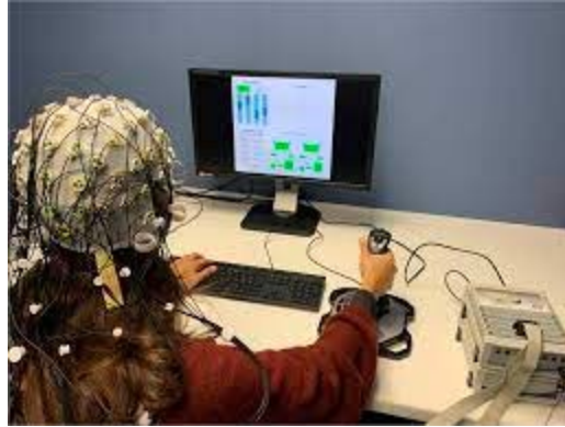
Figure 3. An individual controls the external device using brain activity (Hinss et al. 2023)
