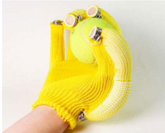
Figure 3. Pneuact developed by MIT which utilizes PAM to aid in finger rehabilitation.
