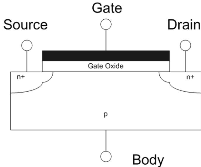
**Figure 2.** Basic component diagram of a field effect transistor
