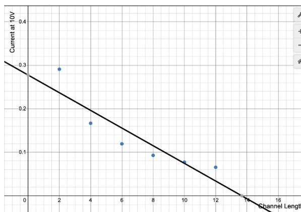
**Figure 9.** Channel length vs current at 10V for reduced graphene oxide
