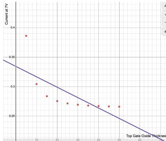
**Figure 8.** Top gate oxide thickness vs current at 7V for reduced graphene oxide
