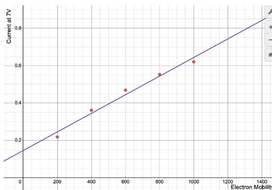
**Figure 11.** Electron mobility vs current at 7V voltage for doped graphene
