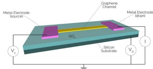
**Figure 16.** Diagram of a potential future graphene-based transistor.
