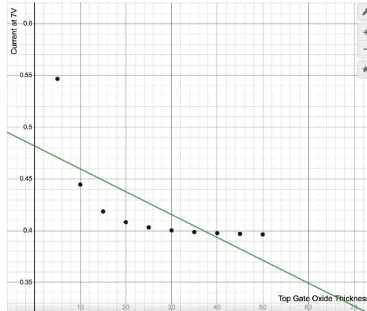
**Figure 13.** Top gate oxide thickness vs current at 7V for doped graphene
