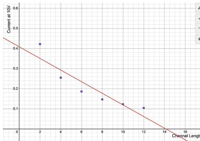
**Figure 14.** Channel length vs current at 10V for doped graphene
