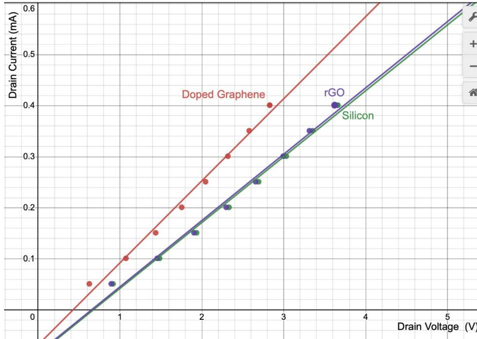
**Figure 15.** Comparisons between the drain voltage vs drain current graphs for doped graphene, reduced graphene oxide (rGO), and silicon.
