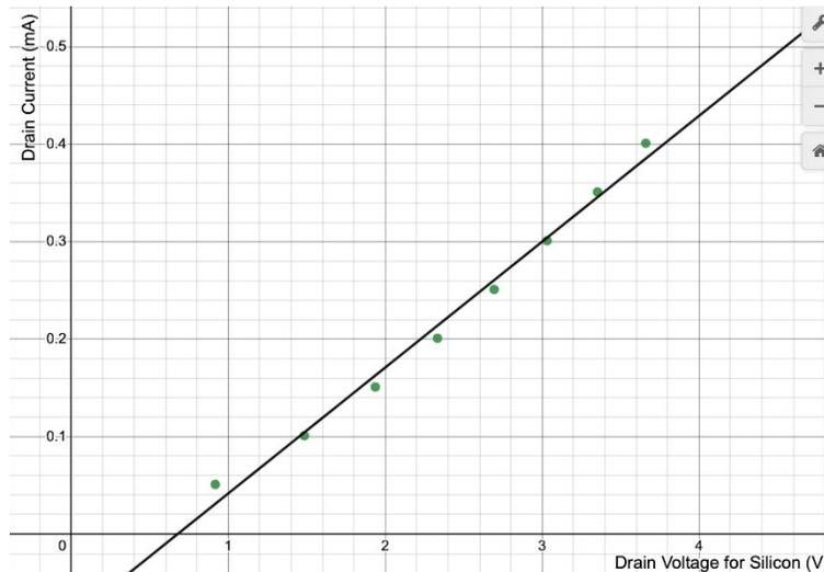
**Figure 5.** Drain voltage vs drain current for silicon
