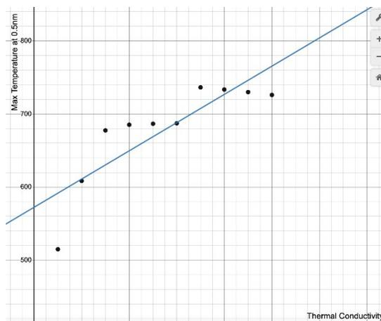
**Figure 12.** Thermal conductivity vs maximum temperature at 0.5 nm position for doped graphene.
