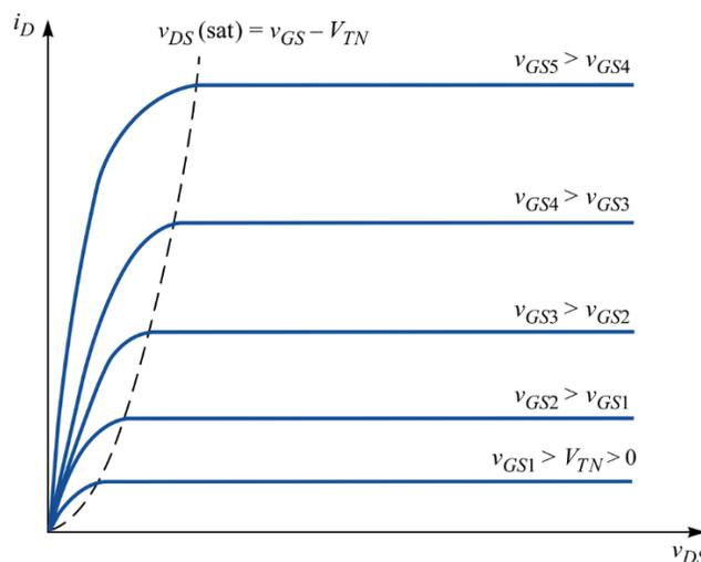
**Figure 3.** Voltage drops from source to drain (V) vs drain current (A) for an ideal FET at varying gate voltages [5]
