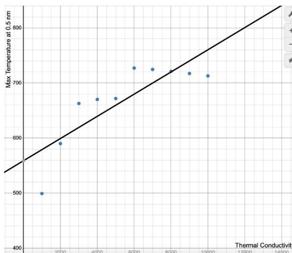
**Figure 7.** Thermal conductivity vs max temperature at 0.5nm position for reduced graphene oxide
