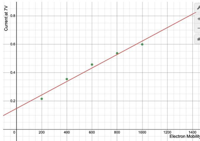
**Figure 6.** Electron mobility vs current at 7V for reduced graphene oxide
