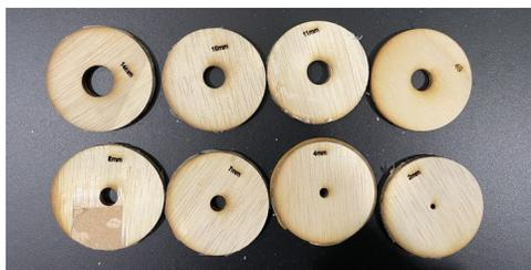
**Figure 3.** the lids of the silo used in the experiment, with orifices made by laser cut and sizes designed by Adobe CAD(Author's Own)
