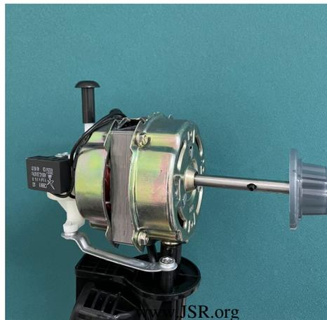
**Figure 8.** the motor used in the experiment(dismantled from a fan motor)
