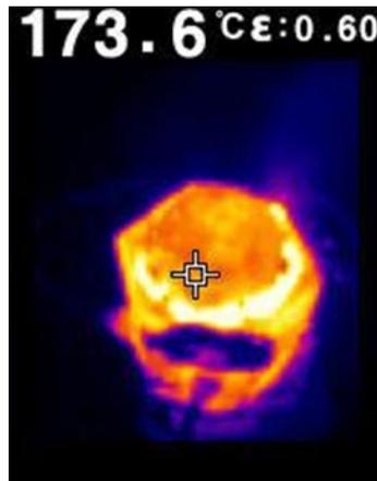
*First Test Thermal Camera Combustion Chamber*
