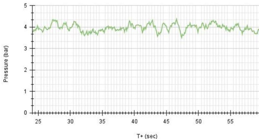
In this test, the pressure was relatively consistent and kept around 4 bar of pressure.
