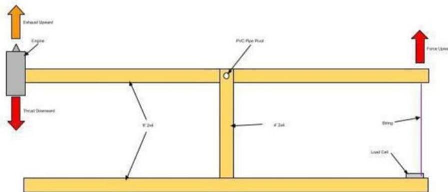
Figure 23. Diagram of the testing apparatus
