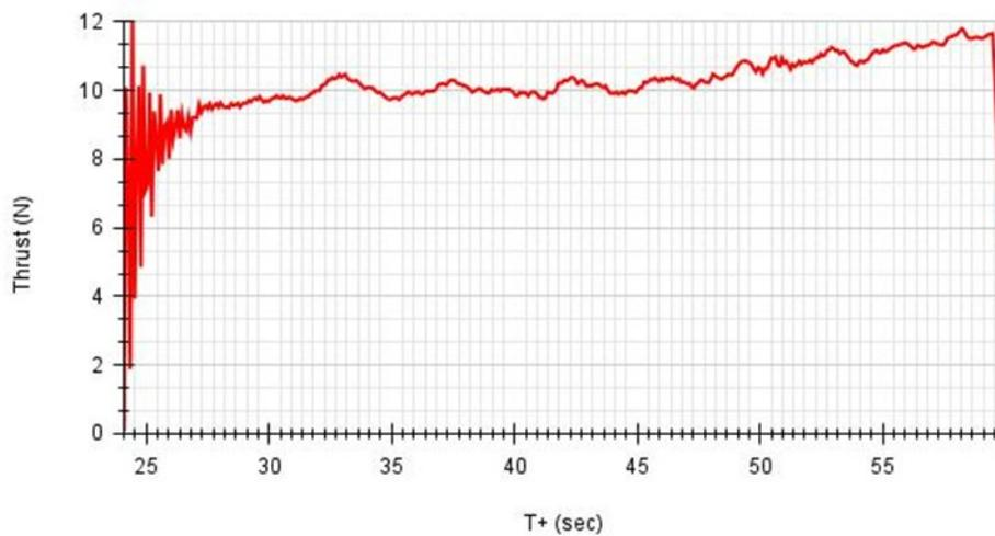
The stand slightly oscillated initially during this test, then settled to a steady rise in thrust over the 30-second test. The thrust started at around 9 newtons and ended at around 12 newtons with an average of around 10.5 newtons.
