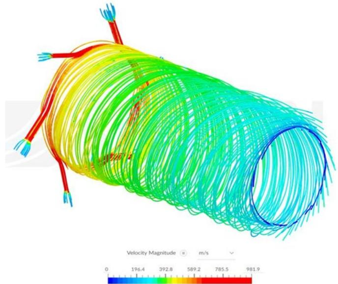
**Figure 11.** The CFD simulation of all six vortex generators
