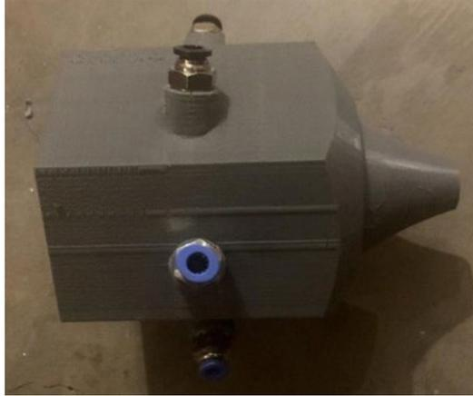
**Figure 21.** The 3d printed nozzle
