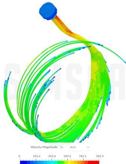
**Figure 10.** The CFD simulation of a single vortex generator
