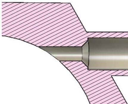
**Figure 8.** The oxygen inlet venturi
