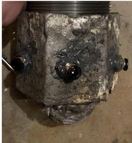
**Figure 22.** This is the nozzle I cast out of aluminum
