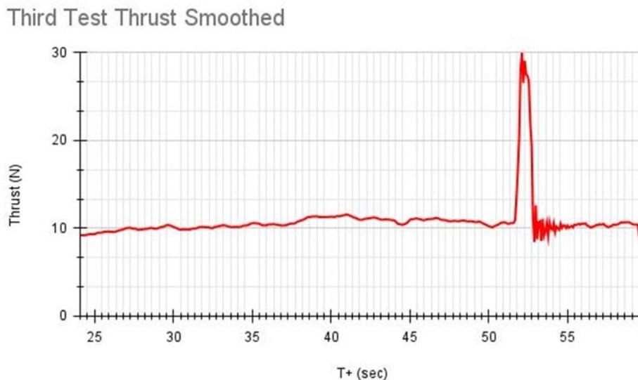
This test started very well with a constant 10 newtons of force until around T+ 50 seconds, when there seemed to have been an anomaly. After the spike caused by the anomaly, the thrust returned to around 10 newtons for the rest of the burn.
