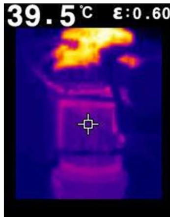
In these photos taken by a FLIR thermal imaging camera, one can see the difference in the temperatures between the combustion chamber and the nozzle.
