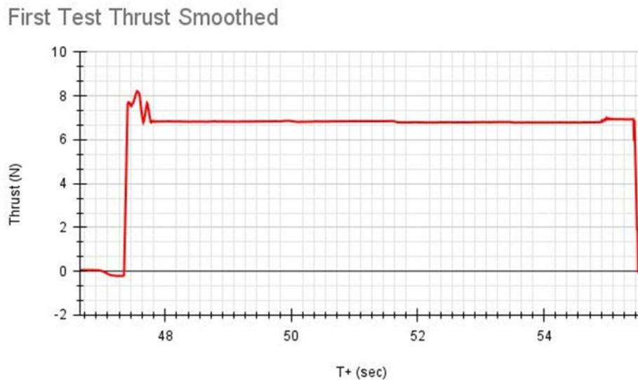
The thrust curve can be clearly seen in both the smoothed and the raw thrust data. With a spike at the start, the thrust over the next 8 seconds is extremely consistent, with an average of around 7 newtons of thrust.
