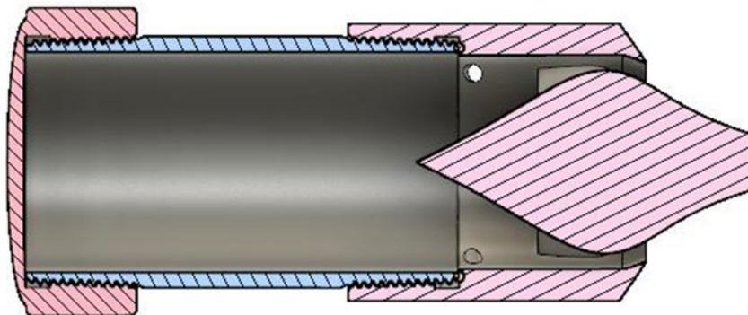
**Figure 12.** A side cut of the rocket engine with the plug aerospike
