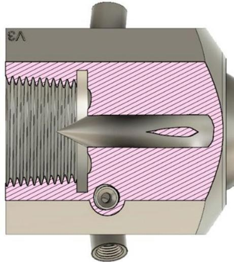
**Figure 15.** A cutaway view of the size of the nozzle to see the airfoil shape
