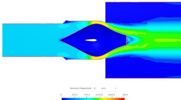
**Figure 16.** Sideview of the optimal aerospike at 1 atm of pressure
