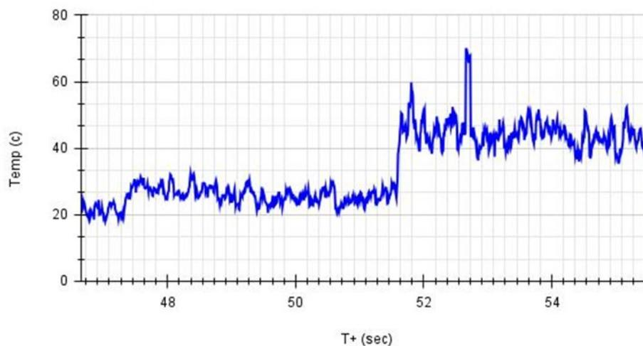
Even with this averaging, the temperature is still quite noisy. However, an overall trend can be seen. About halfway through the burn, the temperature jumped from around 20°C to around 50°C, where it stayed constant for the rest of the burn.
