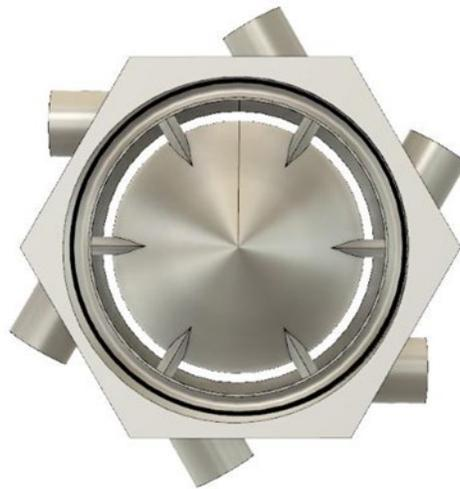
**Figure 14.** A back view of the nozzle to see the six pylons
