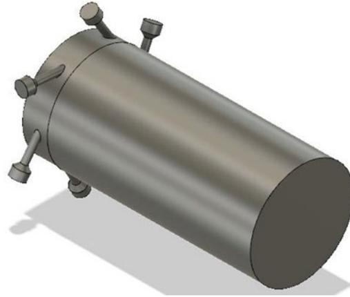
**Figure 9.** The negative of the combustion chamber
