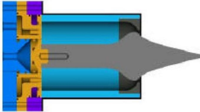
**Figure 13.** The type of plug aerospike detailed in Johnson et al's research
